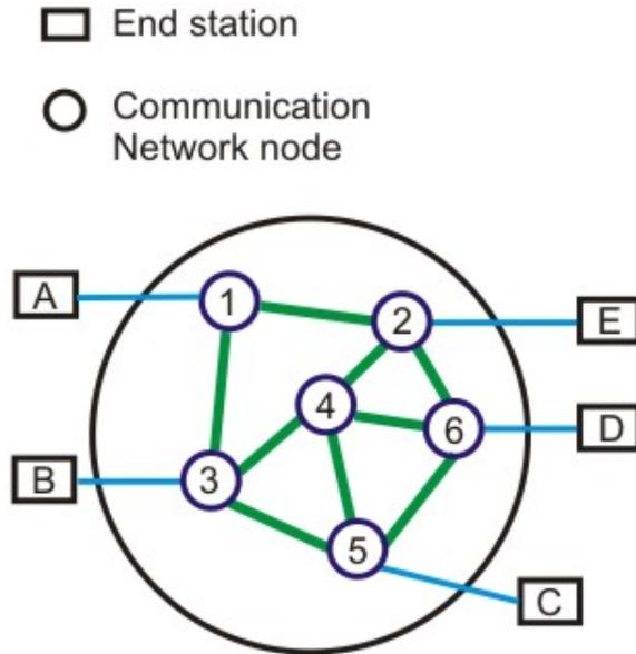
**Figure 1.1.4** *Communication network based on point-to-point communication*
